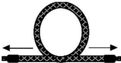
Unrolling a hose by dragging it by the ends creates stress as well as exceeding the bend radius.
