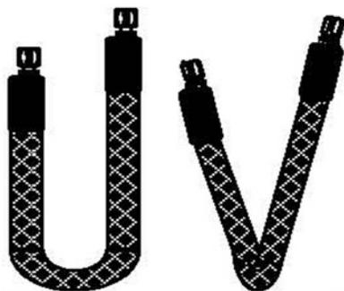
Heated hoses are often destroyed by torsional motions caused by improper installation.
