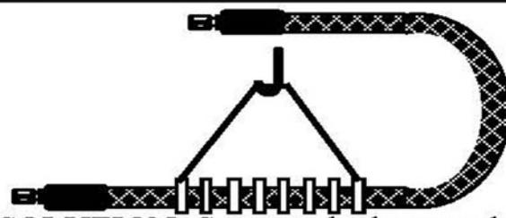
SOLUTION: Support the hose and ensure that the hose is long enough. Do not enclose the hose.
