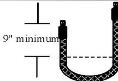
SOLUTION: Plan for a straight piece of hose about 9 - 10 inches before bending.
