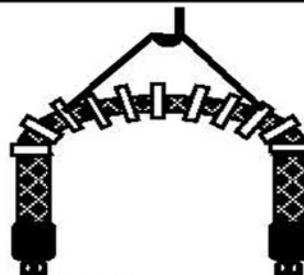
SOLUTION: Use a support with the proper bend radius. Do not enclose the hose.
