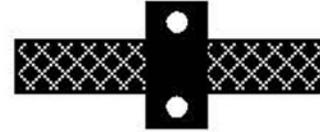
SOLUTION: Use mounting hardware that is large enough to accommodate Hose O.D. with out crushing. Sufficient ventilation is required in mounting hardware.
