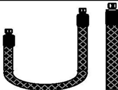
SOLUTION: Make sure that the axes of the heated hose run parallel and the motions are always on one and the same level.
